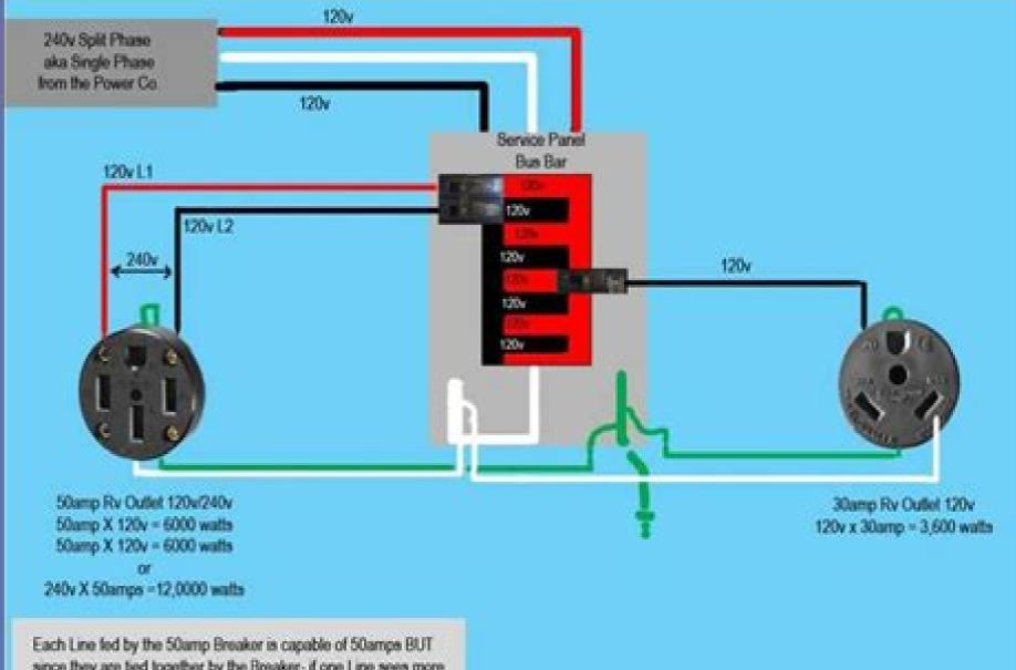
Each Line fed by the 50amp Breaker is capable of 50amps BUT since they are fied together by the Breaker- if one Line sees more than 50amps the Breaker trips both lines
