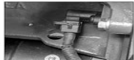
3.11b Engine crankshaft position sensor and multi-plug
