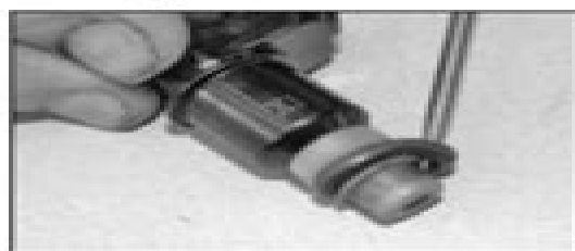
10.18a Remove the O-rings
