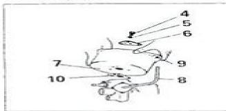
20. With unit body held in bench vice, place a new gasket (10) in position. Locate the vacuum cylinder (7) on gasket (10) with vacuum pipe (8) in new rubber grommet (9). Fit plate (6) and using bolts (4) with new copper washers (5); TIGHTEN BOLTS FINGER TIGHT ONLY.
