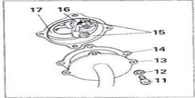
Fit spring plate (17) and lever guide (16).
