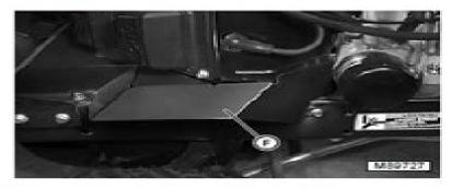
Remove exhaust heat shields (F) from both sides of engine.
