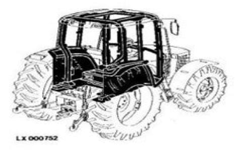
Remove the operator's cab.
