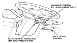
2002-03 models: Unplug the cable reel 4P connector from the driver's airbag 4P connector.
