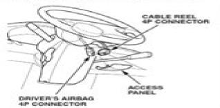
NOTE: When unplugged the driver's airbag connector is automatically shorted.
