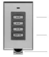
Press left side to turn on, right side to turn off modules set to Unit Codes 1, 2, and 3 on Housecode A (the default setting). Then press and hold left side to brighten or right side to dim.
