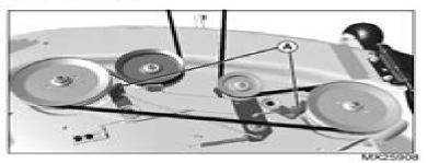
3. Remove left and right belt shields, and adjust two blade brakes (A).
