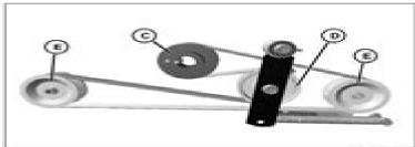
Hydraulic Pump Drive Belt Tensioner Assembly Repair
