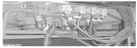
AT17652-UN: XY300 - 2-Pin Connector for EHM III Shut-Off Solenoid Valve Y300 XY300 - 2-Pin Connector for EHM III Shut-Y300 - EHM III Shut-Off Solenoid Valve Off Solenoid Valve Y300
