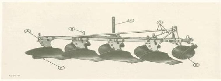
A-Safety-Trip Standard D-Mast Braces B-Coulter Shank E-Rolling Coulter C-Support Stand F-Rear Landelde
