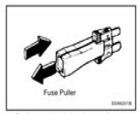
4. Replace the blown fuse by pressing a new fuse of the same rating into place. The fuse should be a snug fit. If it is not, have the fuse clip repaired or replaced by a Hyundai dealer. If you do not have a spare fuse, you may be able to borrow a fuse of the same or lower rating from an accessory you can temporarily get along without (the radio or cigarette lighter, for example). Always remember to replace the borrowed fuse.
