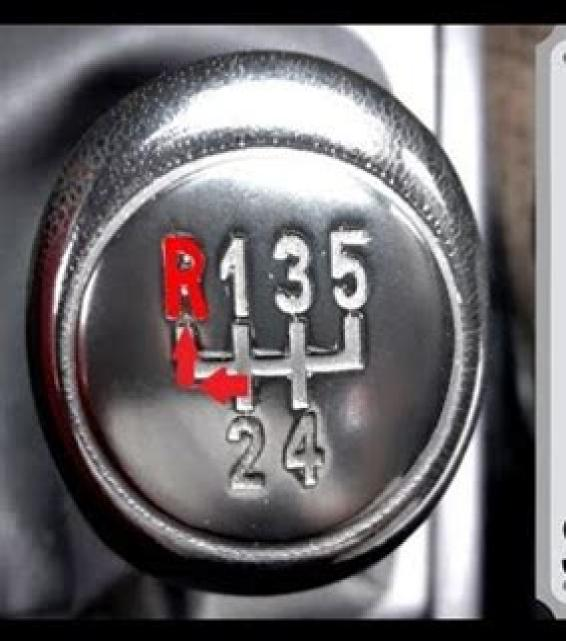
**HOW TO** FIND REVERSE **GEAR** ON ANY STICK SHIFT CAR
