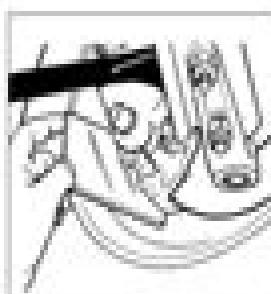
16.1 Checking the front disc pad wear using a screw.
