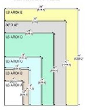
Anchi tectural sheet sizes are based upon a 36" x 48" sheet, and proportionally smaller sizes. In addition to the above, the 24" x 42" sheet size is commonly accepted as a standard size.
