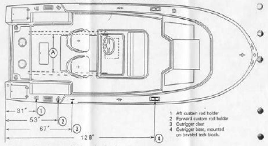
Showing locations of custom rod holders and uutrigger bases.
