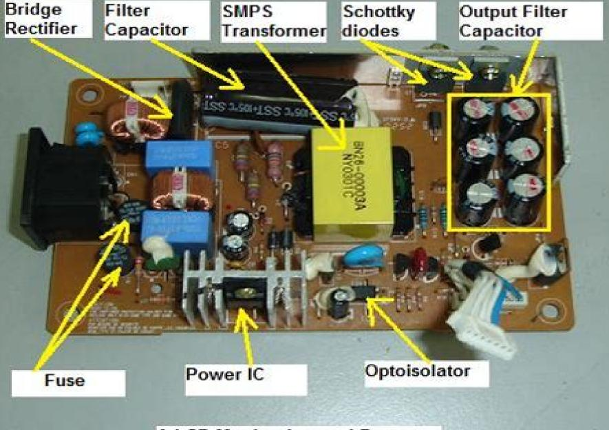
A LCD Monitor Internal Power Supply Board
