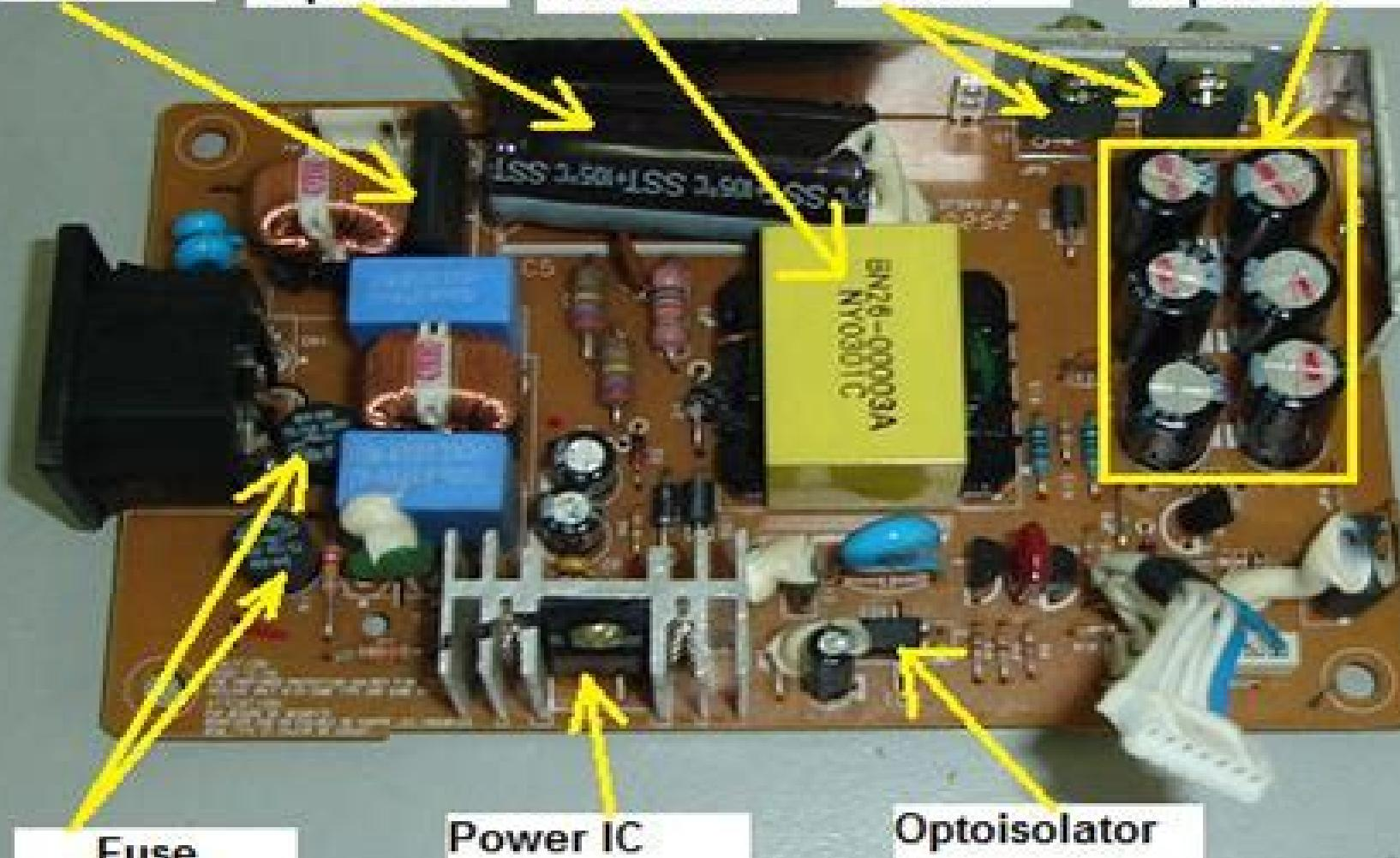
A LCD Monitor Internal Power Supply Board
