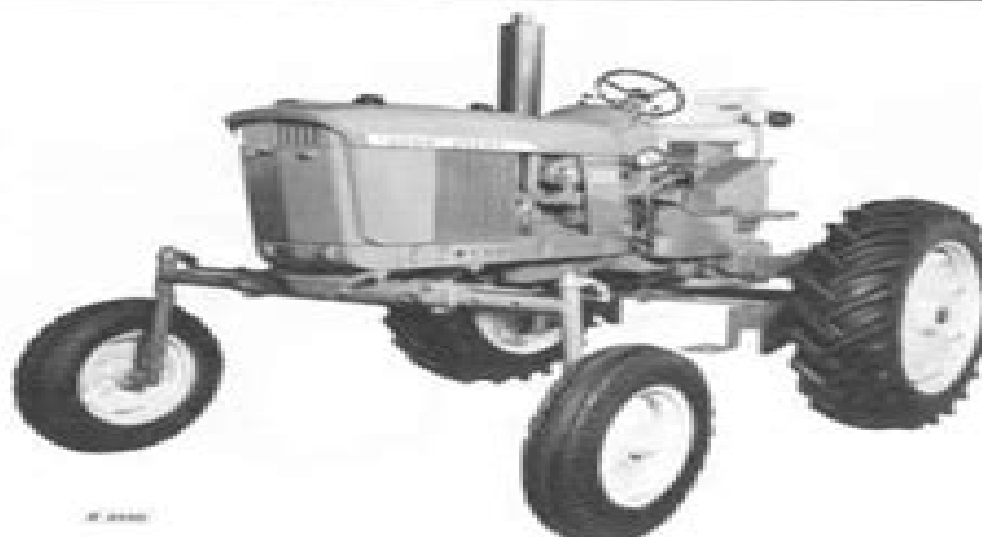
Fig. 10-5-3—Right-Hand View of John Deere 3020 Hi-Crop Tractor with Gasoline Engine
