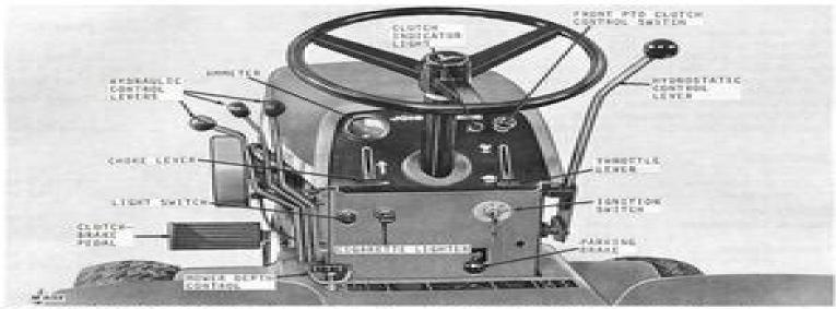
PTO CLUTCH CONTROL SWITCH - This pushpull switch engages or disengages the electromagnetic clutch to drive mower and front-mounted equipment.
