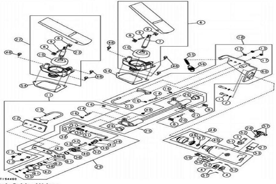
Brake Pedal and Linkage
