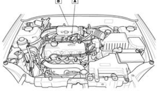
A Positive Crankcase Ventilation Valve (PCV valve)
