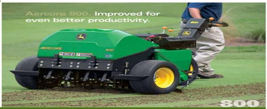
Bring on the large greens and tees. With the changes we've made to the walk-behind Aercore 800, you'll be getting more done in less time. With a new 25-hp Kohler engine, the Aercore 800 delivers increased power to the coring head and traction drive systems. It also allows for lower engine rpms on entry and exit. increasing hole quality. And a mechanical transmission reduces hydrautics on your greens.
