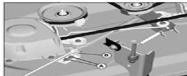
3. Loosen nuts (A) and move cable bracket (B) away from the center of mower deck to tighten belt tension. Move bracket until almost all slack is out of cable but cable is not too tight. Tighten nuts.
