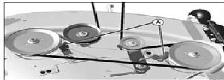
3. Remove left and right belt shields, and adjust two blade brakes (A).
