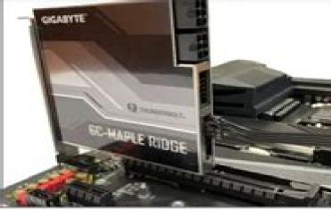
Step 4: Connect one end of the Thunderbolt\* header cable (5-pin) to the 5-pin Thunderbolt\* header on the GC-MAPLE RIDGE add-in card.
