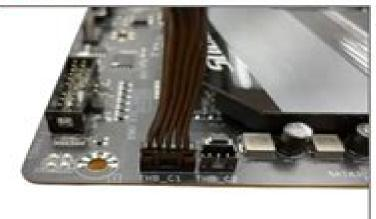
Step 5: Connect the other end of the cable to the Thunderbolt" add-in card header (Note 1) on the motherboard.
