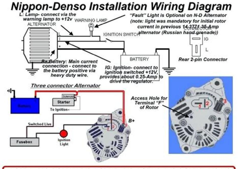
Grounding the "F" terminal gives "full-field" for testing.
