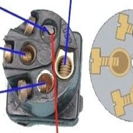
Terminal 2 is covered with thin plastic. Twist the plastic and remove it before using terminal 2
