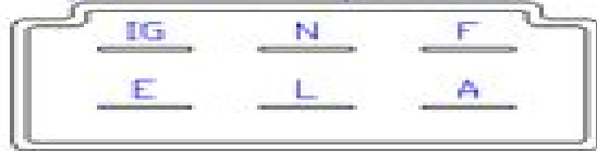
Pin lay-out of 6-pole connector
