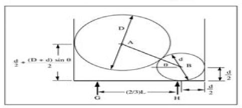
From the above diagram and the free body diagram for C, the forces G and H can be obtained.
