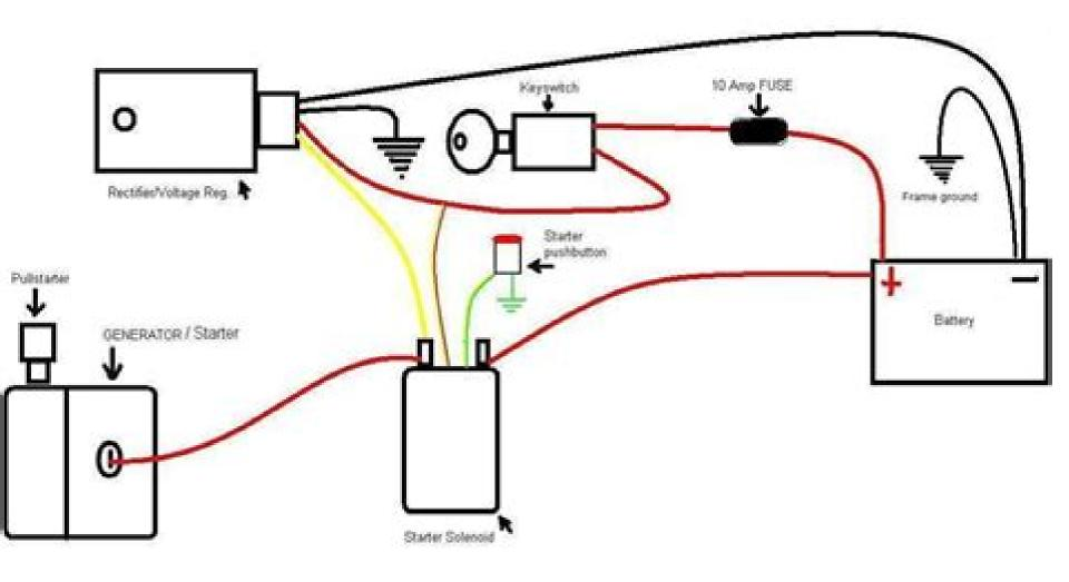
2 Stroke Wiring Diagram Starter/Charging System
