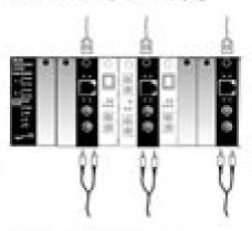
The AutoCrass<sup>to</sup> feature allows either straight-through or crossover twisted-pair copper cable to be used when connecting the C/E-TX-SX-02 to a 10/1008ASE-TX device.
