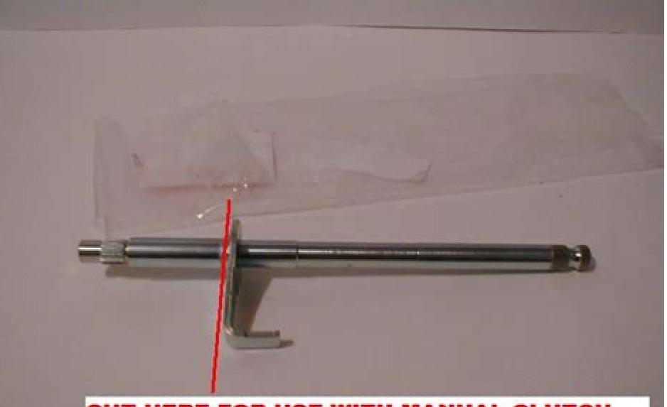
CUT HERE FOR USE WITH MANUAL CLUTCH COVERS, THIS SHAFT IS ABOUT AN INCH LONGER THAN THE STD MANUAL TYPE SHAFT
