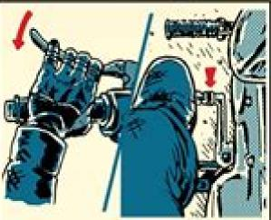
2. Squeeze in the clutch lever and press down on the gear shift lever to reach 1st gear.
