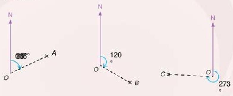
The true bearings of A, B and C measured from O are  $065^{\circ}$ ,  $120^{\circ}$  and  $273^{\circ}$  respectively.
