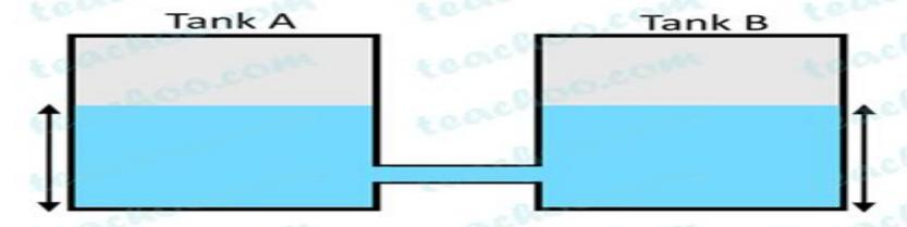
Since Tank A has higher water level, So, water **will flow** from Tank A to Tank B
