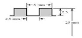
(b) Thread depth = 2.5 mm Ans. Width at pitch line = 2.5 mm Ans.  $d_m = 22.5$  mm  $d_r = 20$  mm I = p = 5 mm Ans.
