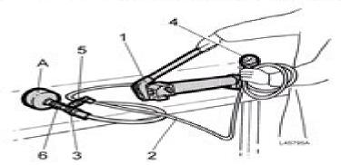
Figure 1 Checking removed accumulator
