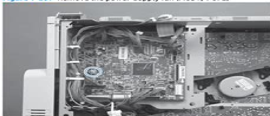
Figure 1-297 Remove the power-supply fan (M651; 1 of 2)
