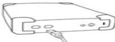
Figure 3 1394 Interface Cable Hook-up
