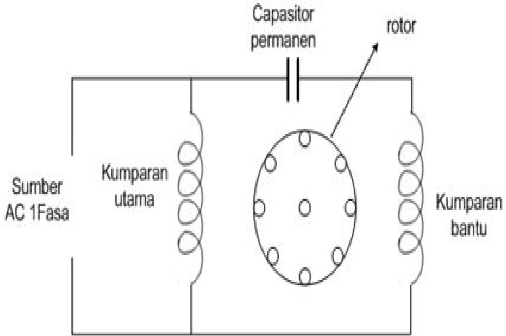
Gambar 04. Motor running kapasitor
