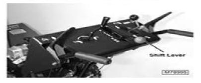
3. Move shift lever into "6" (6th gear) position.
