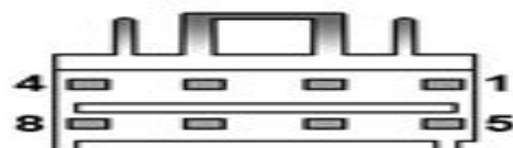
8 pin GM 89047379 (19115652) amplifier wiring harness connector
