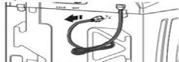
Firmly grasp power cord plug and pull to free from rear panel. Gently place power cord over console to allow free access to back of washer.
