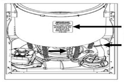
Note: Sticker indicating this machine has been modified with a "High Torque" service transmission and Seal kit 2101868. Placement of sticker is necessary when converting from the old transmission to the new "High Torque" transmission.
