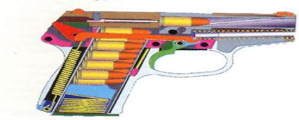
The ignited powder gas drives the bullet forward through the barrel and simultaneously drives the slide and barrel backwards. After about 3/16" (5 mm) the barrel is cammed down by the assembly pin and releases the slide to travel back extracting the case. On it's way back, the slide is gradually slowed down by the recoil springs.
