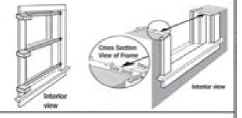
To determine the height of the new window, measure between the top of the sill, just behind the stool, and the underside of the head jamb. If necessary, remove the stops for accurate measurement.
