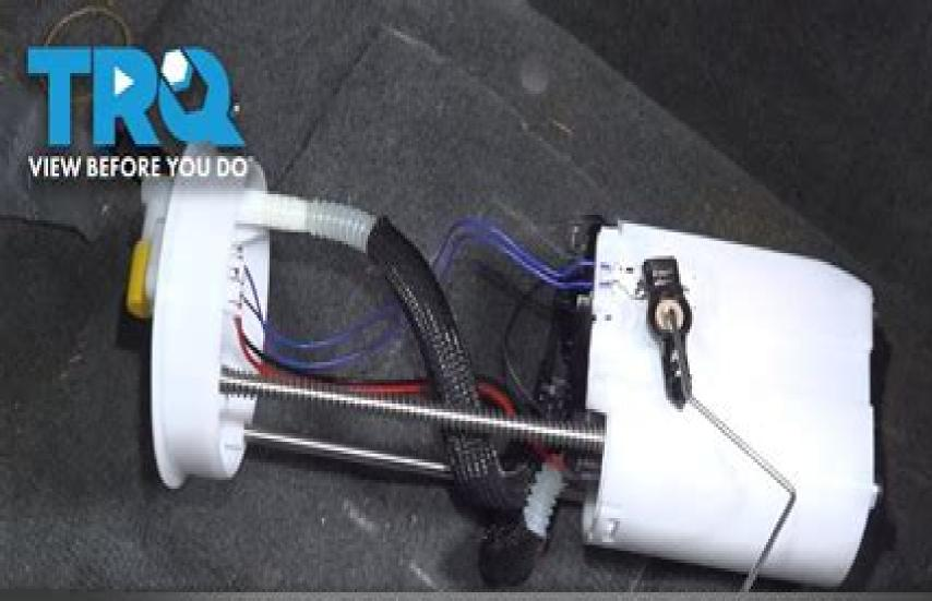
HOW TO REPLACE FUEL PUMP ASSEMBLY 2003-2008 HONDA PILOT
