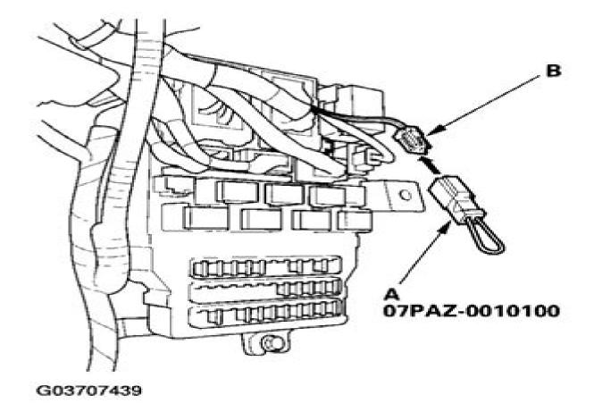
Fig. 34: Connecting SCS Service Connector To Yellow MES 2P Connector Courtesy of AMERICAN HONDA MOTOR CO., INC.
