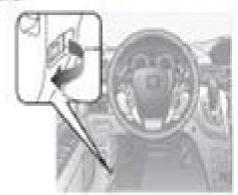
Locate the hood latch lever, slide the lever, and lift up the hood
